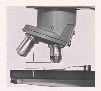
Since all objectives are designed for use with cover glass thickness of 0.18mm, make it a practice to use this proper thickness cover glass over all preparations. It is significantly important to recognize that too thick a preparation may make it impossible to focus onto its deepest detail with the 100X, or possibly with a 43X or 45X objective, because of the relatively short working distance of high powered objectives.
