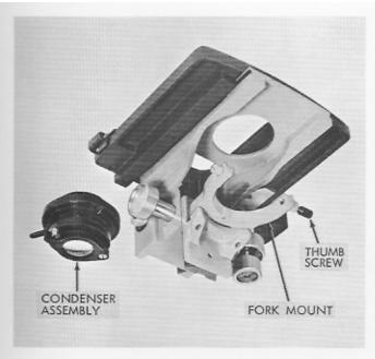
Figure 16. Removal of Condenser Assembly
