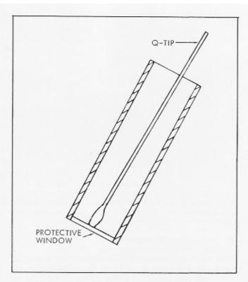
Figure 30. Cleaning Protective Window
