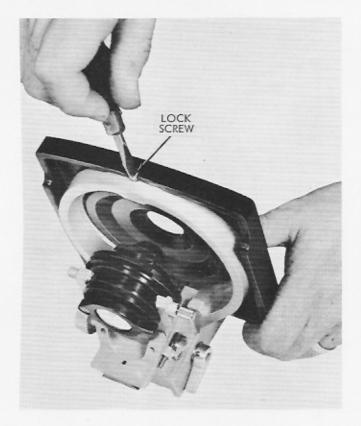
Figure 14. Removal of Simple Stage
