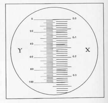
Figure 8. Calibration of Micrometer Discs
