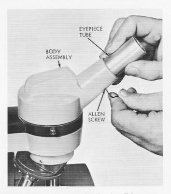
Figure 29. Removing Eyepiece Tube
