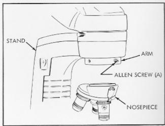
Figure 31. Removing Nosepiece
