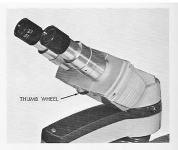
Figure 20. Interpupillary Distance Adjustment
