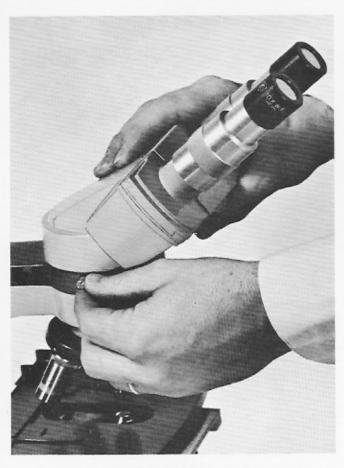
Figure 1. Attaching Binocular Body to Stand
