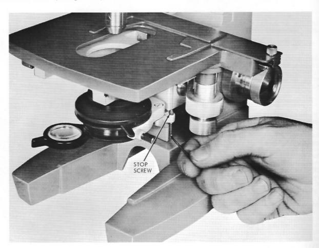
Figure 15. Adjusting Condenser Heights
