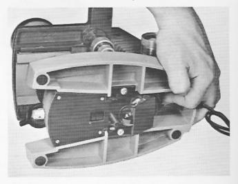
Figure 26. Changing Lamp in "In-Base" Illuminator
