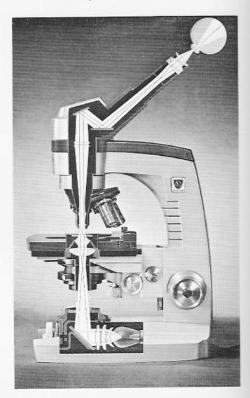
Figure 5. Infinity Corrected System
