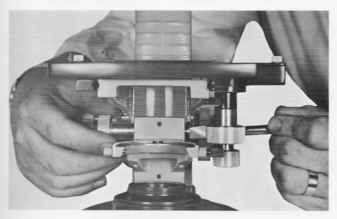
Figure 18. Adjustment of Focusing Tension
