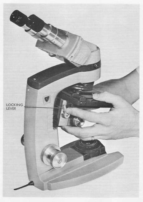
Figure 12. Removal of Stage Assembly
