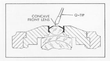
Figure 28. Cleaning Front Lens of #1078 45X Objective
