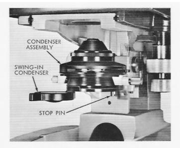
Figure 19. Auxiliary Swing-in Condenser
