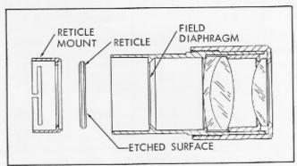
Figure 7. Wide Field Eyepiece
