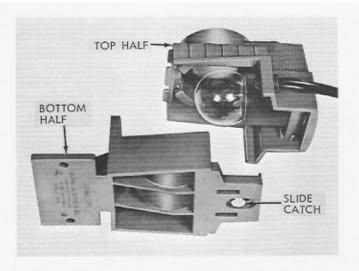
Figure 24. Changing Lamp in 'On-Base" Illuminator
