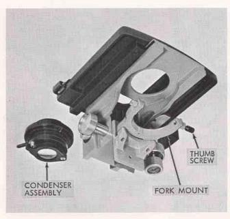
Figure 16. Removal of Condenser Assembly
