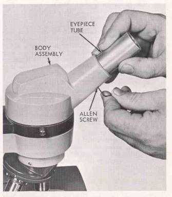
Figure 35. Removing Eyepiece Tube
