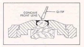
Figure 34. Cleaning Front Lens of #1023 40X Objective
