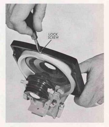
Figure 14. Removal of Simple Stage
