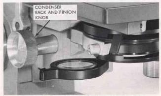
Figure 30. Condenser Rack and Pinion Knob
