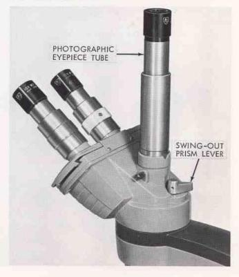
Figure 21. Trinocular Body
