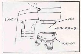
Figure 37. Removing Nosepiece
