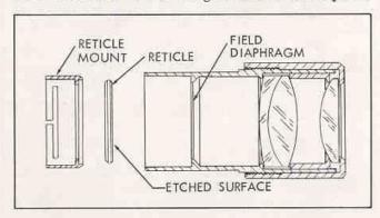
Figure 7. Wide Field Eyepiece
