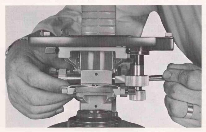
Figure 18. Adjustment of Focusing Tension
