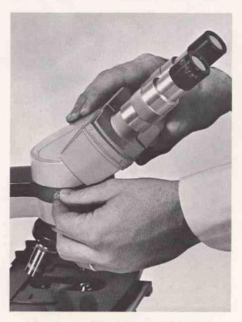
Figure 1. Attaching Binocular Body to Stand
