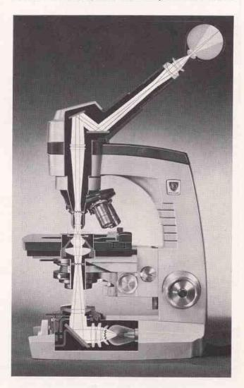
Figure 5. Infinity Corrected System
