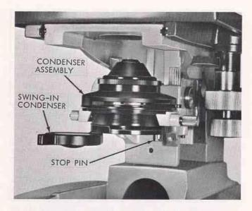
Figure 19. Auxiliary Swing-in Condenser
