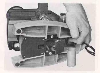
Figure 26. Changing Lamp in "In-Base" Illuminator
