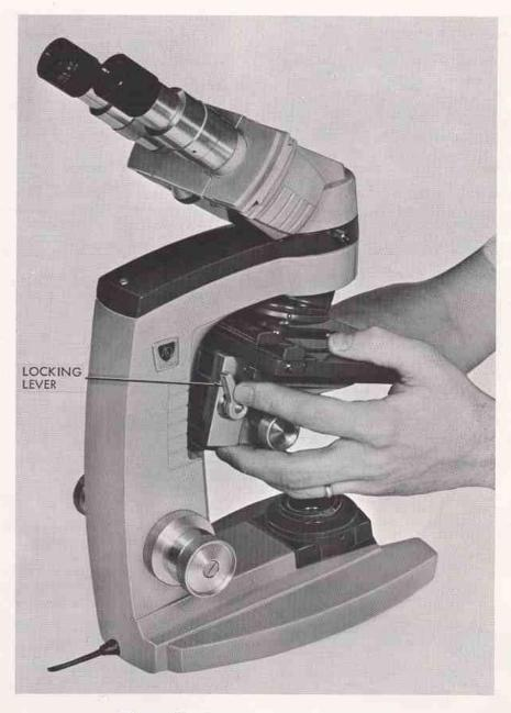
Figure 12. Removal of Stage Assembly
