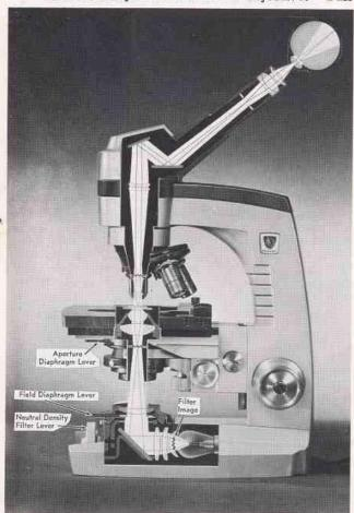
Figure 25. Infinity Corrected Optics and Koehler Type Illumination
