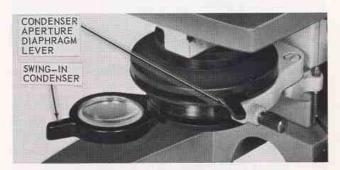
Figure 29. Substage Condenser and Aperture Diaphragm
