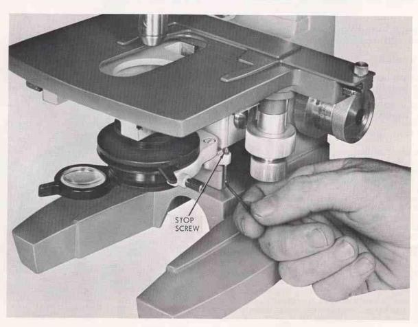
Figure 15. Adjusting Condenser Heights
