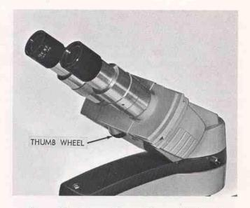
Figure 20. Interpupillary Distance Adjustment
