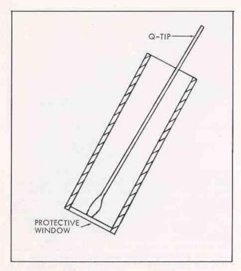
Figure 36. Cleaning Protective Window
