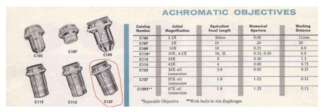
For American Optical Series 10/20 microscopes, the funnel stop needed is Catalog No. 214-79, for the 100X Cat. 1079 oil immersion objective.
