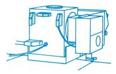
• The connection cable of the automatic camera with the multiple plug is connected to the associated connector at the rear of the microscope. There are three female connectors: one for a camera on the left, the second for a camera on the right, and the third for a top-mounted automatic camera.
