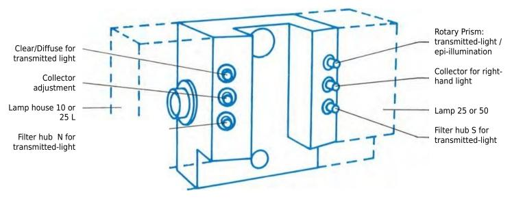
On the mirror house 2, two bulbs of your choice can be attached, e.g., the halogen lamp on the left, and the lamp house 25 or 50 on the right. This allows:
