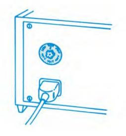
• Operating voltage: the control unit is normally set to 220V. When switching to a different voltage, the inner head of the voltage selector is pushed in and removed after a quarter-turn of the screw counterclockwise. With a coin or screwdriver blade, you can then move the voltage selector to the desired voltage.
