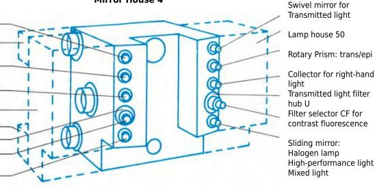
On the mirror-house 4, a halogen lamp can be used for both transmitted and reflected light and can be supplemented by two high-power lamps; e.g. on the left, lamp house 25, and on the right, lamp house 50. The mirror knobs allow (by simply switching):
