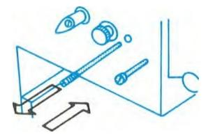
**c)** Remove the red locking screw for the beamsplitter prism and replace with the supplied 32mm long screw.
