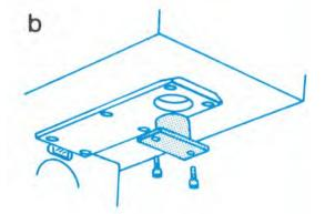
**b)** Remove the red protector in the relay housing.
