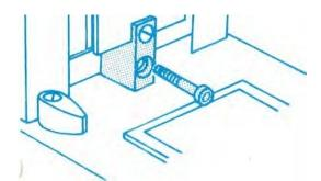
**d)** Remove the red protector on the focus rack, after unscrewing the hex bolt and the slotted screw. Withdraw the protector after the rack is slightly raised. Replace the slotted screw.
