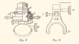
is open in front. This unit goes definitely into place, and when centered with the centering screws the whole optical train of the microscope is in perfect alignment.
