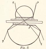
of the objective and the cover glass. It is assumed that the object is embedded in a medium having the same index as the slide and the cover glass. It is seen that the ray goes through the system without any deviation between the two curved surfaces, due to the fact that the oil has the same index as the slide, cover glass and the two
