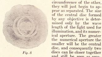
and still be seen as separated. It has already been pointed out that the size of the central disc does not vary with the corrections 34 which determine the quality of the definition. Evidently then, the resolving power does not depend in any way on the definition.
