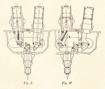
venience of the device immediately appeals to the research worker. Figure L shows the position of the parts when both eyepieces are used. Figure M shows the same parts in the position assumed when but one eyepiece is in working position.
