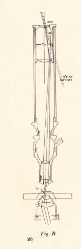
of proper focus of the instrument. This should be avoided. It is not always easy to know that the instrument is properly focussed. To test for this, gaze vacantly out of a window at a distant object and then look quickly into the microscope. If the image is blurred at the first instant and gradually clears, the instrument is not properly focussed and it should be refocussed.
