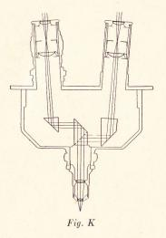
the objective. The  $45^{\circ}$ surface of one of these prisms is semi-platinized to reflect half the light to one side, and allow the other half to pass through to be reflected in the opposite direction by another 45° reflecting surface. These two beams of light are again reflected upward, each to its evepiece, by prisms located directly below the eyepieces and moving with them. The eyepieces are movable to and from one another to accommodate different inter-
